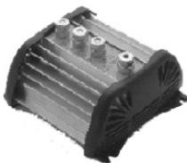
Battery isolators separate electrically each battery to avoid that the battery with the highest charge drains into the one with the lower charge. During the charging phase, the isolator allows the preferential recharging of the battery bank most in need. The casing is made of aluminum, with wide cooling fins designed to disperse heat efficiently. They are supplied complete with nuts, washers and wire housings for connection, as well as directions for correct assembly.
